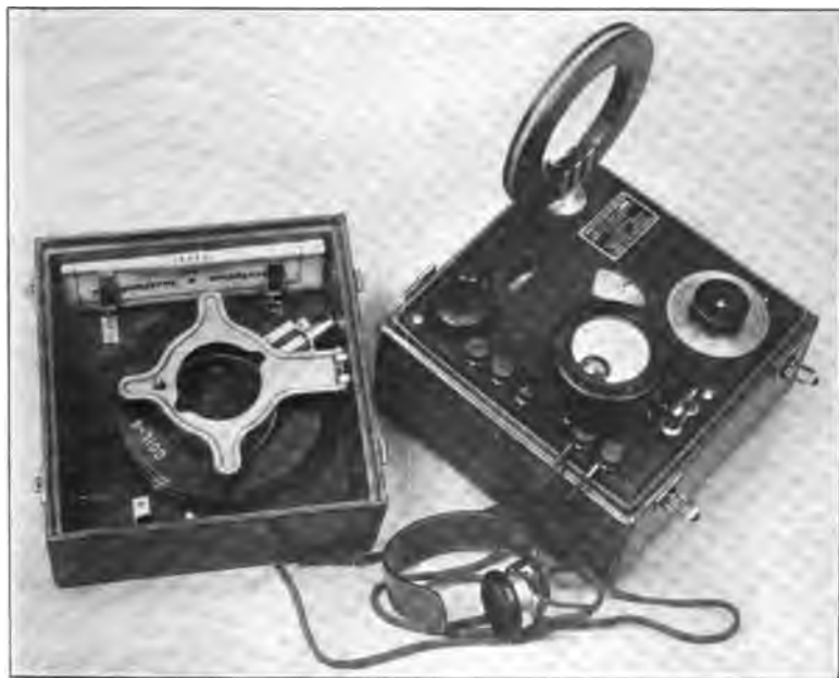
Plate 1. —Bureau of Standards Kolster decremeter and wavemeter type D. Wave length range by means of four interchangeable coils, 70 meters to 3000 meters; decrement range 0 to 0.3.
